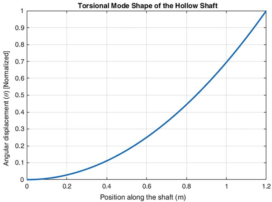
Figure 4. The mode shape of the composite shaft for 319.42 Hz.
