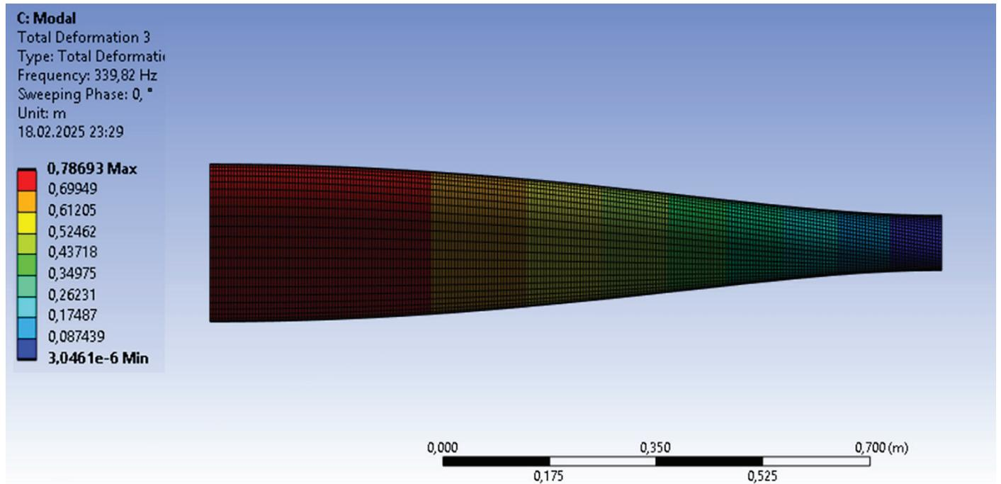
Figure 3. The mode shape of the composite shaft obtained with ANSYS Modal Analysis.
