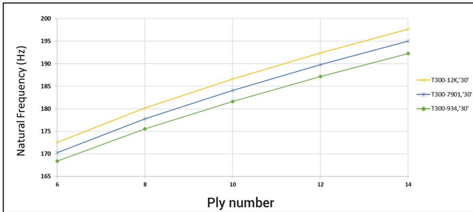
Figure 8. Natural frequencies with different material at ply angle  $\pm 30$ .
