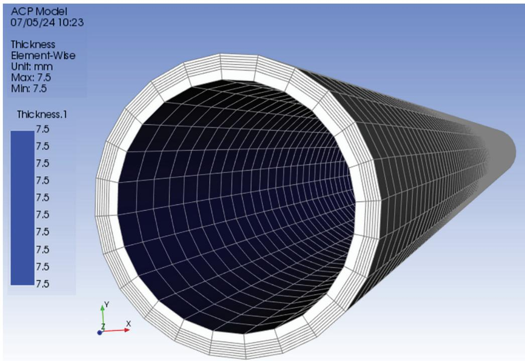
Figure 2. Details of the drive shaft with ANSYS ACP Module
