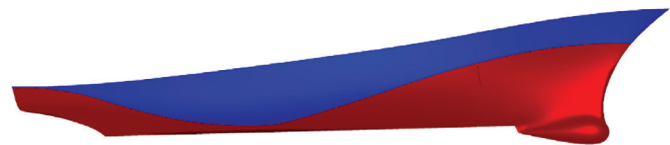
Figure 2. View of the DTMB 5512 when the ship is on the wave trough.
